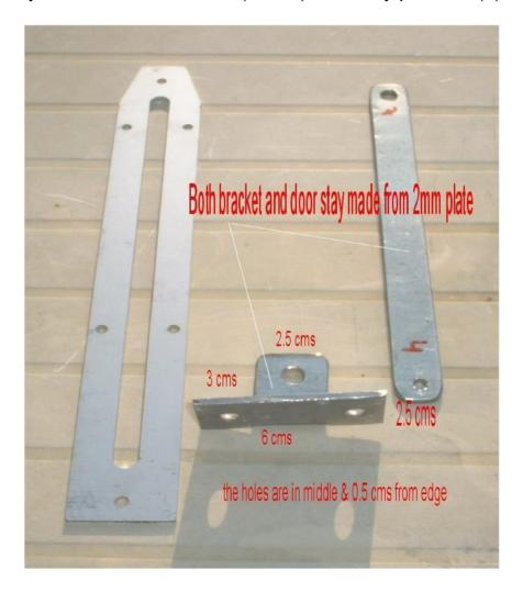
I then recessed into the wood sufficient depth to take the bracket and bolt heads and drilled the retaining holes. The retaining holes pass through the remaining timber to a side chassis plate that becomes the main strength of the whole project, ie. the bracket is bolted to the chassis.
